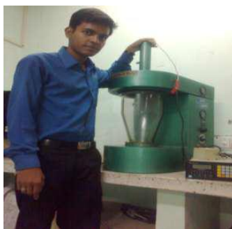
Fig. 1: Fluidized bed drying system 7
